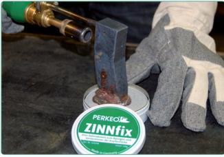
**ZINNFIX** is a new kind of cleaning stone, whereby solder bits can be cleaned far quicker and without any effort required at all. And it produces no aggressive acidic fumes either...
